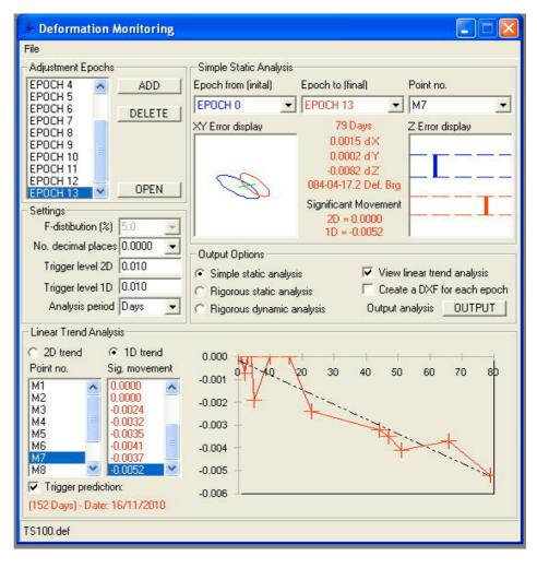
With our own least squares adjustment, error propagation and analysis computer software we can determine if any deformation has occurred and the magnitude, velocity and direction of the movement. This analysis can be delivered to the client as a stand-alone document or embedded into a drawing as text with isopachite contours to visually describe the deformation.
